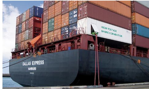
Figure 2.5: Containerised cable management system at the aft of the vessel.
