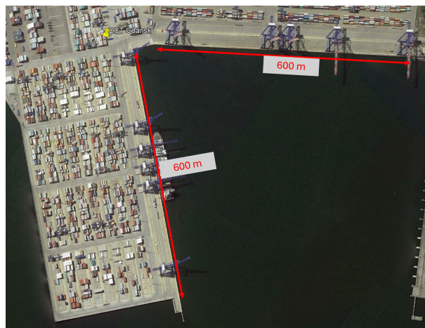
Figure 5.6: Quay layout of the Baltic Hub terminal in Gdansk that is similar to the quay configuration of Scenario 4.
