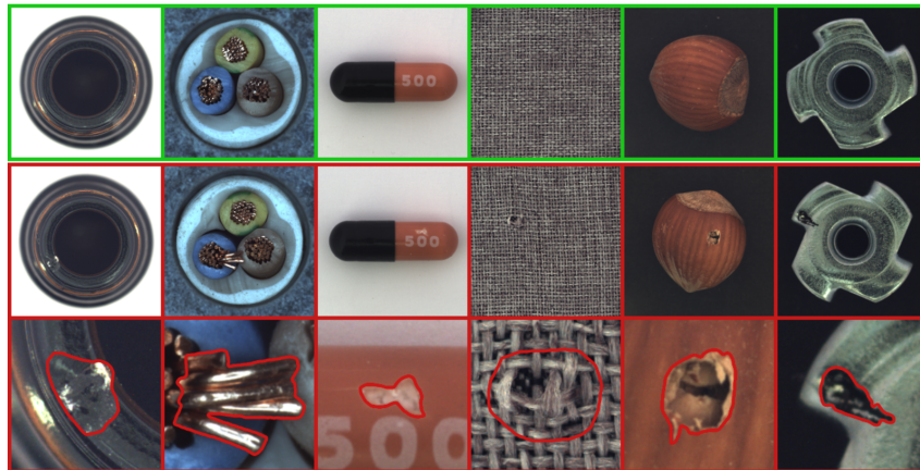
Figure 8: The image categories in the MVTec AD dataset contain normal samples (top), defective samples (middle) and segmentations (bottom).
