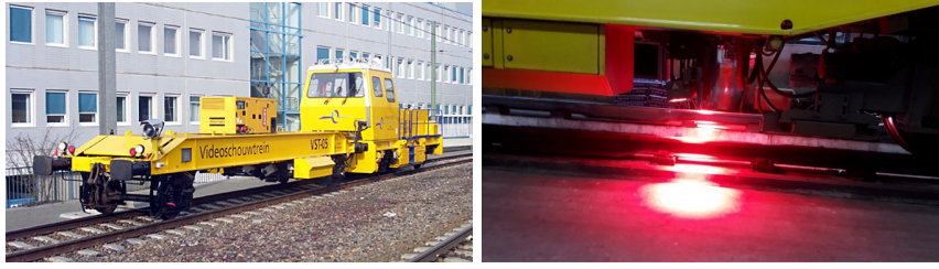
Figure 2: The video inspection train equipped with line scan camera equipment.
