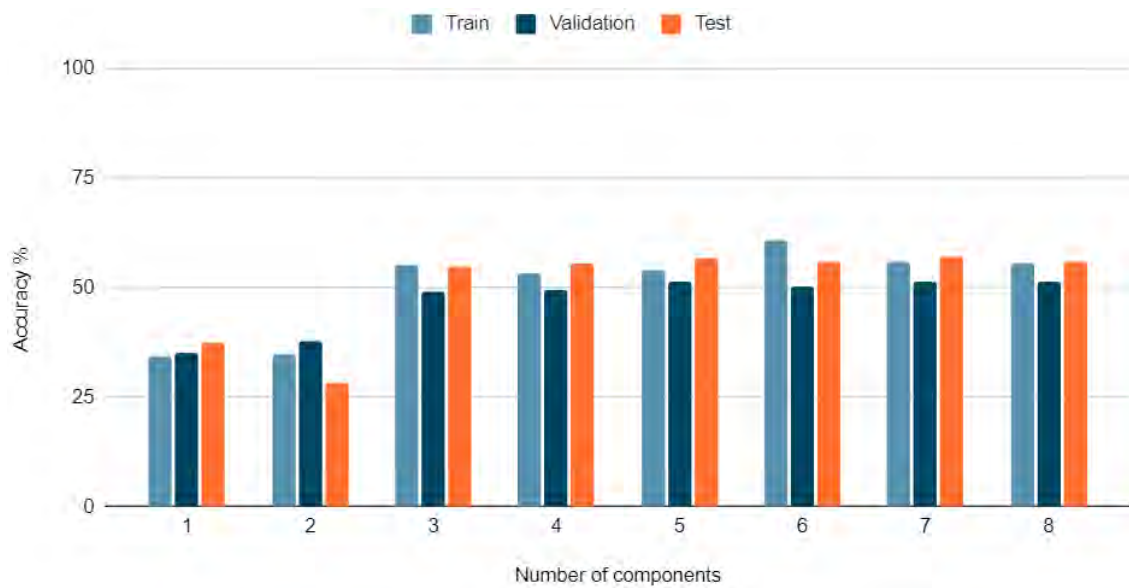
Figure A2: The accuracies of SVM are shown to examine the effects of the amount of CSP components. It can be seen that the validation accuracy is optimal with five components. However, the difference with four components is very small and therefore there is decided to use the simplest model, that also reached the highest accuracy with LR.
