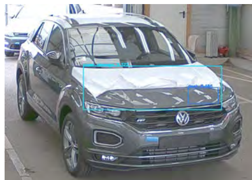
(B) Detected cover damage and detected dent on the bonnet. The left bonnet dent is not detected by the model.
