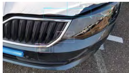
(H) Scratch and Cover damage.
