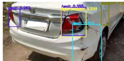
(F) Scratch, Dent, Bent, and Light broken.
