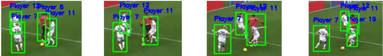
Figure 21: Four subsequent frames, illustrating a failure in re-identification using spatial consistency within the tracking procedure
