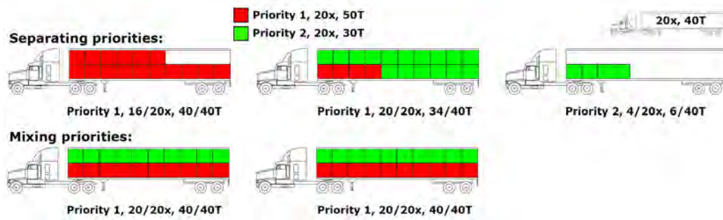
Figure C.1: Example of how allowing priorities to mix can reduce the number of trucks without increasing the number of trucks per priority.
