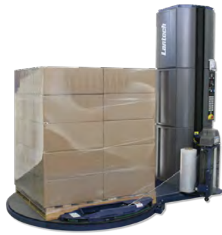
Figure 3.6: Shrink-wrapping of a pallet.
