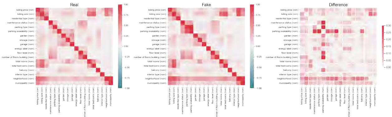
Figure 9.4: The correlation matrices for the empirical sample on which the TVAE submodel is trained (left), synthetic sample generated by the TVAE submodel (middle) and the absolute differences between these matrices (right). A dark red color indicates a high correlation value in the left and middle matrices and a high absolute difference in the right matrix.
