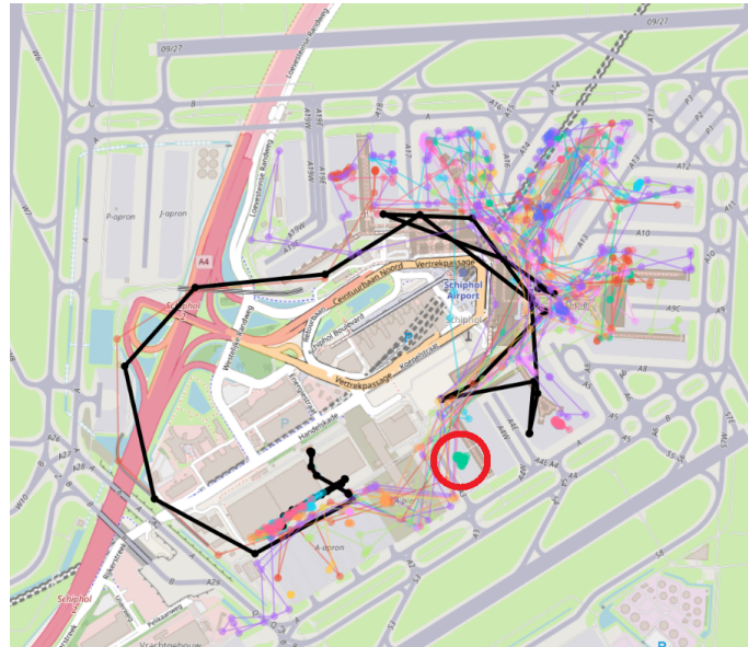
Figure 4.7: Examples of extracted trajectories. Encircled in red, a relatively stationary trajectory can be seen, while the trajectory highlighted in black is shown to go around the premises.
