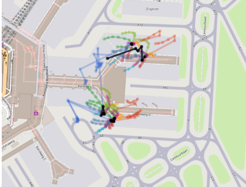
Figure 6.7: Actual and predicted trajectories based on vehicle type 'Trekker 3-wiel'. The black trajectories indicate the true trajectories, whereas each colored trajectory represents a prediction of a given model.
