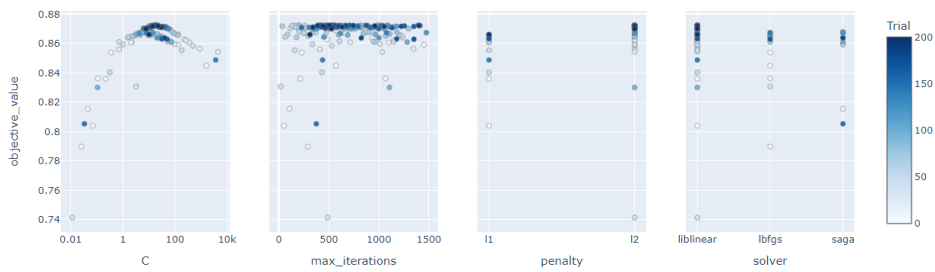
Figure B.1: Hyperparameter tuning experiment of the Logistic Regression model on the Profit & Loss dataset
