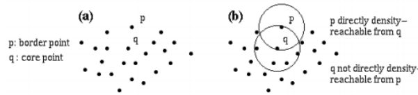
Figure 41: Illustration of how a point p can be directly density-reachable from q while q is not directly density-reachable from p . Image taken from Ester et al. (1996).
