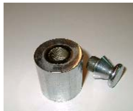
Figure 4: Adjustable weight (example of an artefact that cannot be immersed in water)
