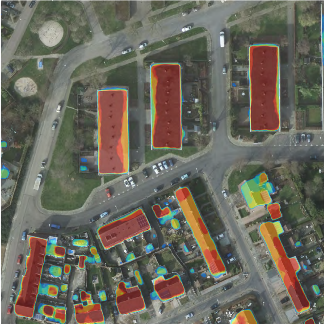
Figure B.9: TTA predictions of ResU-net resolution robustness experiment 1: Trained on 30 cm resolution imagery, tested on 30 cm resolution imagery of Heerlen, The Netherlands. Plotted on 10 cm imagery.
