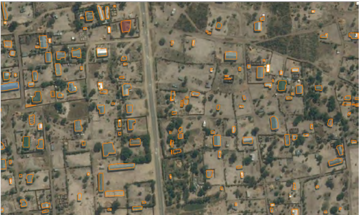
Figure B.4: Sample of vectorized TTA Mask R-CNN predictions on Mongu, Zambia (QGIS screenshot).
