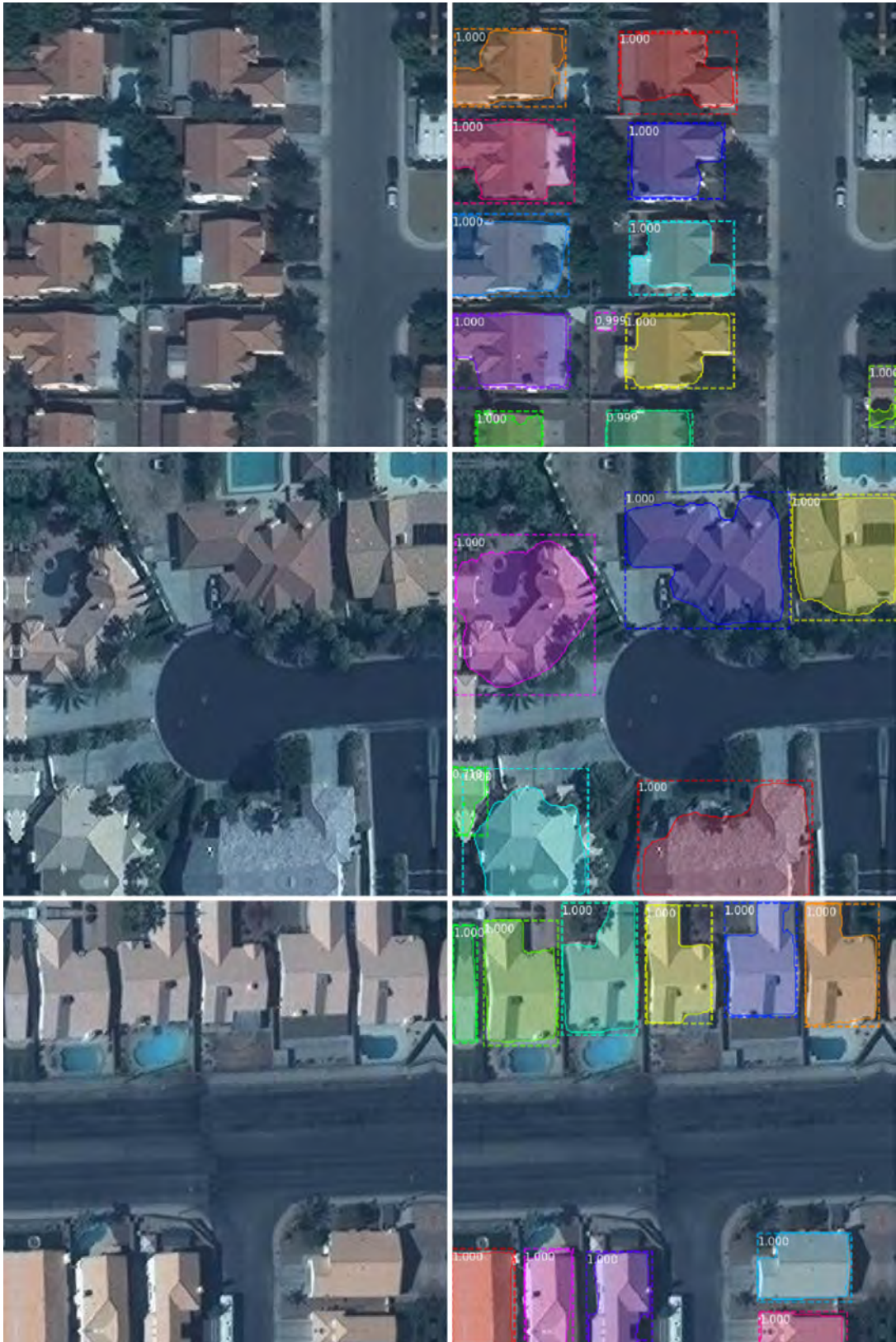
Figure 5.1: Left: Sample images from the crowdAI test set, with reflection-padding applied. Right: Predictions of Mask R-CNN using default parameters. The dotted line visualizes the bounding box, the area within the solid line is the predicted pixel mask and the number represents the certainty of the prediction.
