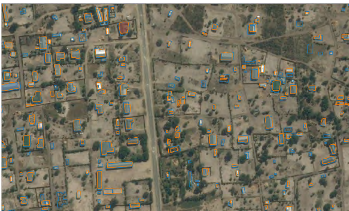
Figure B.6: Sample of vectorized TTA Mask R-CNN predictions (orange outlines) and OpenStreetMap labels (blue outlines) on Mongu, Zambia (QGIS screenshot).
