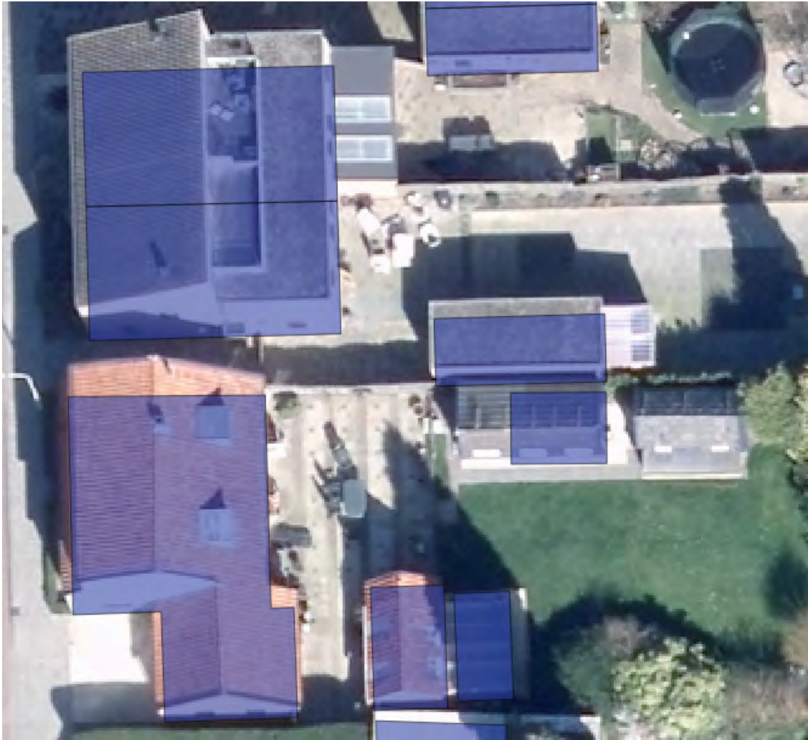
Figure 4.6: This sample image illustrates the quality of Readar’s aerial imagery and ground truth labels. This also illustrates the parallax effect, revealing the building facades.
