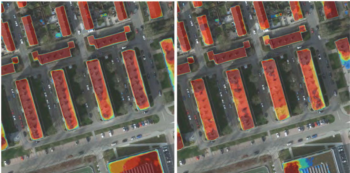
Figure 6.8: Left: A 153.6 by 153.6 meter 10 cm resolution image of Heerlen containing predictions of a model trained and tested on 30 cm imagery. Right: Predictions of a model trained and tested on 10 cm imagery.
