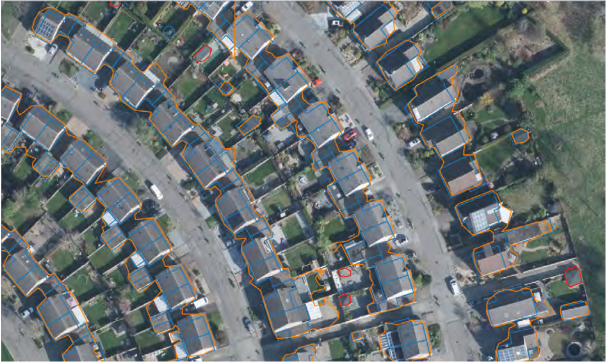
Figure B.15: Vectorized sample predictions on Heerlen by ResU-net. Vectorized sample predictions on Heerlen by ResU-net. An orange outline indicates the prediction overlaps at least one building in the ground truth, red indicates no overlap. Blue outlines are buildings in the BAG or BGT database (QGIS screenshot).
