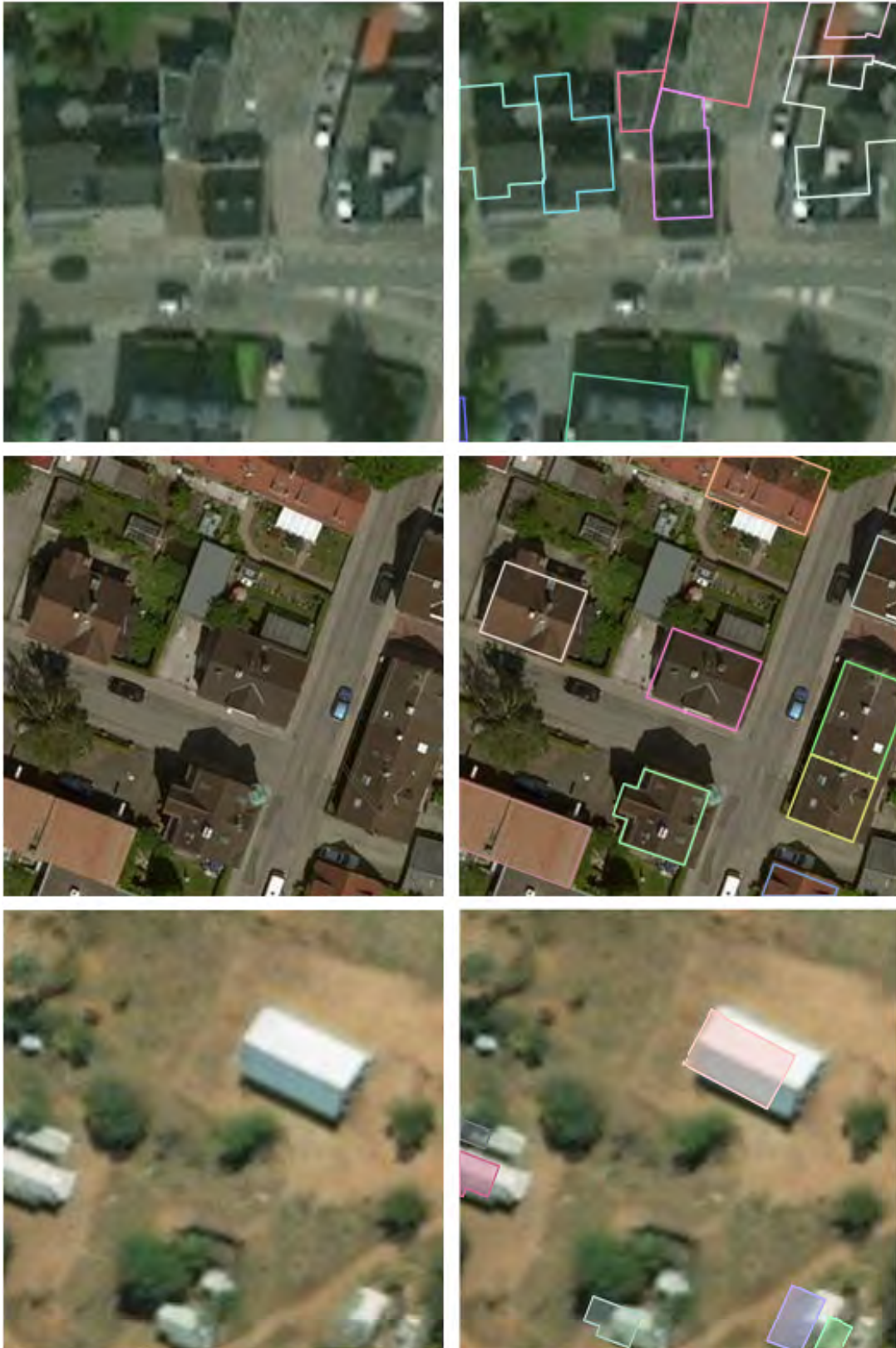
Figure 4.3: Left: Samples from Bing Maps imagery, right: OpenStreetMap building outlines plotted on Bing Maps imagery. Location in descending order: Hulsberg, Limburg, Netherlands, 30 cm resolution - Augsburg, Bayern, Germany, 15 cm resolution - Nsanje, Nsanje, Malawi, 30 cm resolution.
