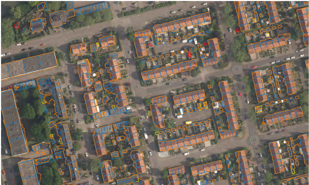
Figure B.14: Vectorized sample predictions on Amersfoort by ResU-net. An orange outline indicates the prediction overlaps at least one building in the ground truth, red indicates no overlap. Blue outlines are buildings in the BAG or BGT database, yellow outlines are manually mapped buildings (QGIS screenshot).
