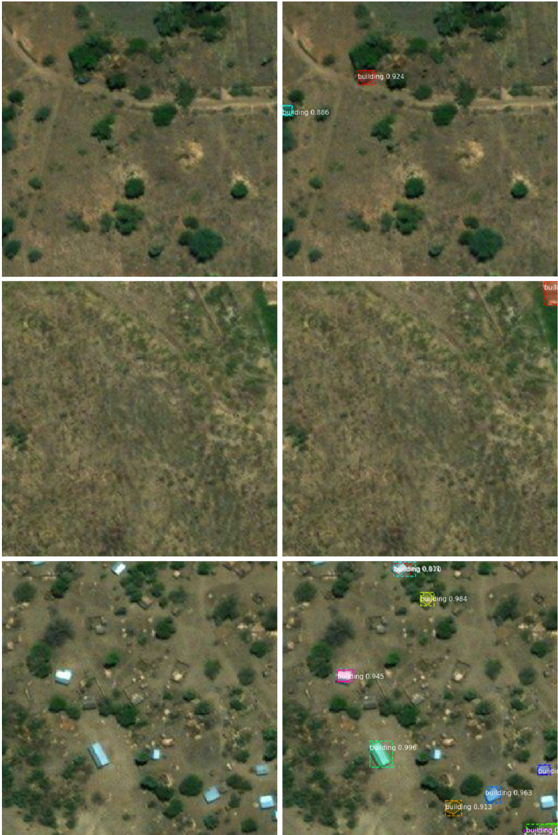
Figure 5.2: Left: Three sample images of 153.6 by 153.6 meters from the 60 cm resolution Bing Maps imagery of the Nsanje region in Malawi. Right: Mask R-CNN predictions on those images. Only predictions with a certainty above 0.5 have been plotted.
