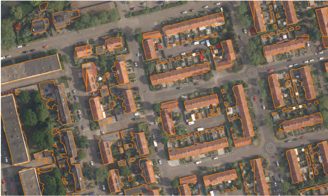
Figure 6.11: Vectorized predictions on Amersfoort. An orange outline indicates the prediction overlaps at least one building in the ground truth, red indicates no overlap.
