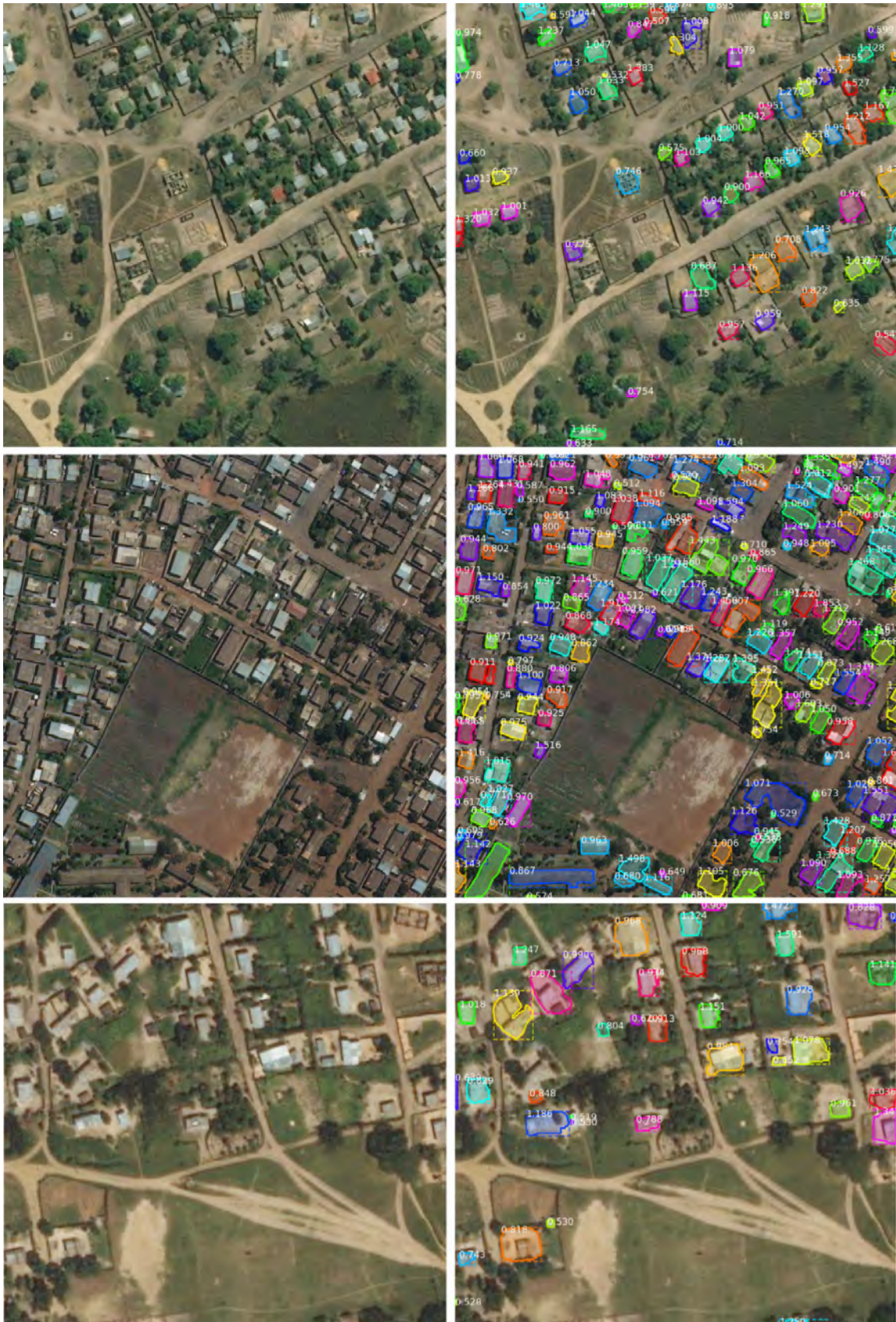
Figure B.2: Left: Samples from imagery of Zambia at 30 cm resolution. Right: TTA predictions of Mask R-CNN on imagery upsampled by a factor of 2.5. Top row: A 307.2 by 307.2 meter sample from Kalabo. Middle row: A 307.2 by 307.2 meter sample from Lusaka. Bottom row: A 230.4 by 230.4 meter sample from Zambezi.
