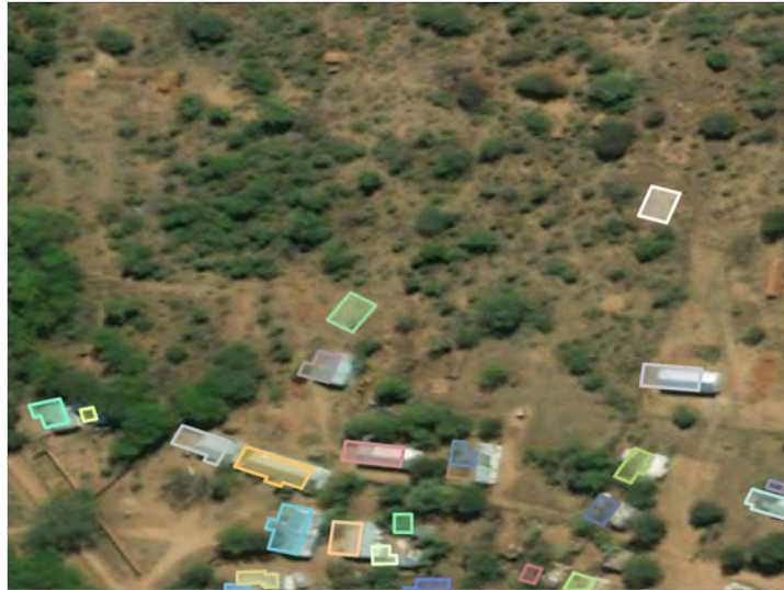
Figure 4.4: Sample from OSM ground truth labels overlaid on Bing Maps satellite imagery of Nsanje at 30 cm resolution. The imagery does not show any buildings belonging to the two most upper instances. There also is a consistent misalignment between the ground truth labels and the imagery.
