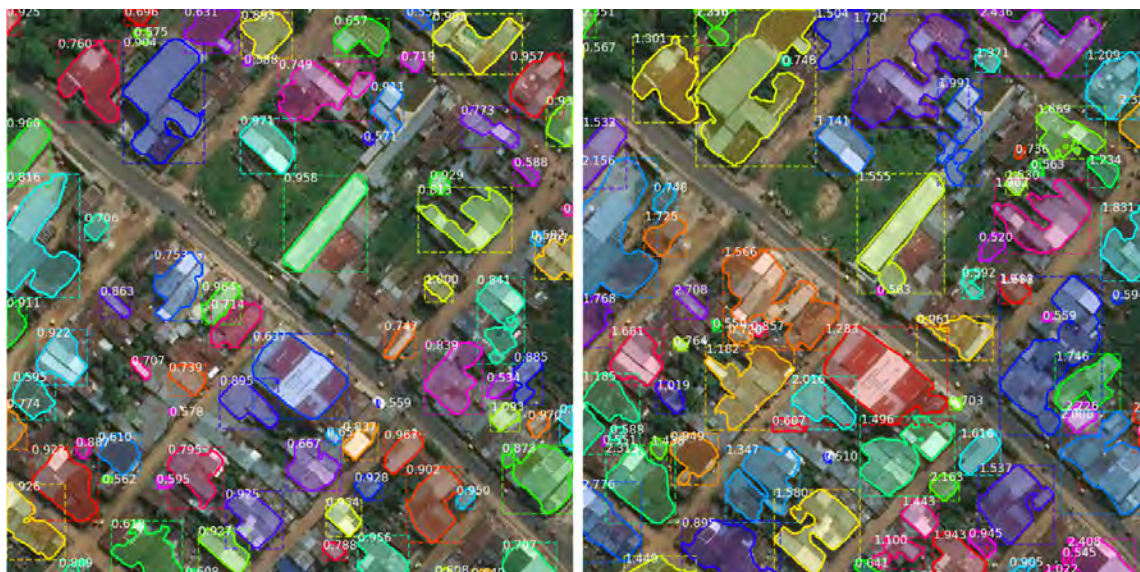
Figure 5.8: Left: TTA predictions with a 0.3 NMS threshold. Right: TTA predictions with a 0.8 NMS threshold.
