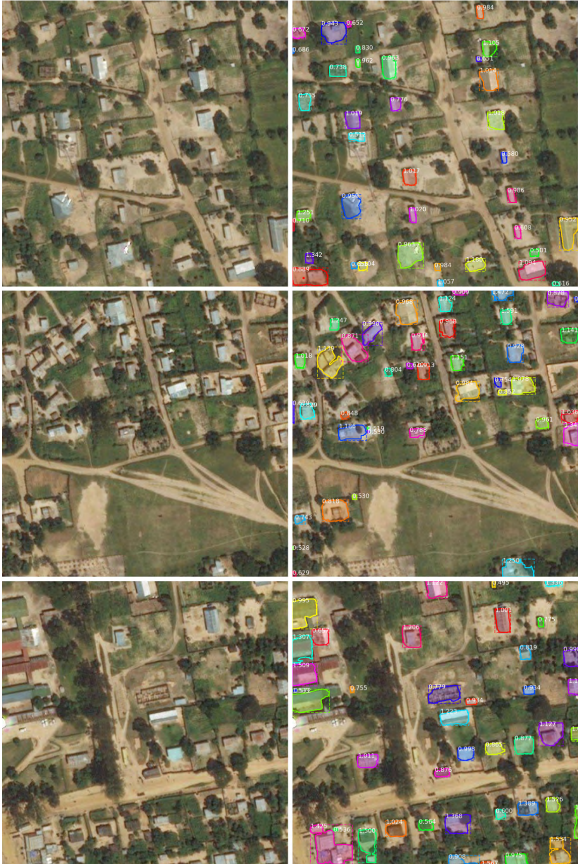
Figure 5.5: Left: Samples of 230.4 by 230.4 meters from imagery of Zambezi at 30 cm resolution. Right: TTA predictions of Mask R-CNN on imagery upsampled by a factor of 2.5.
