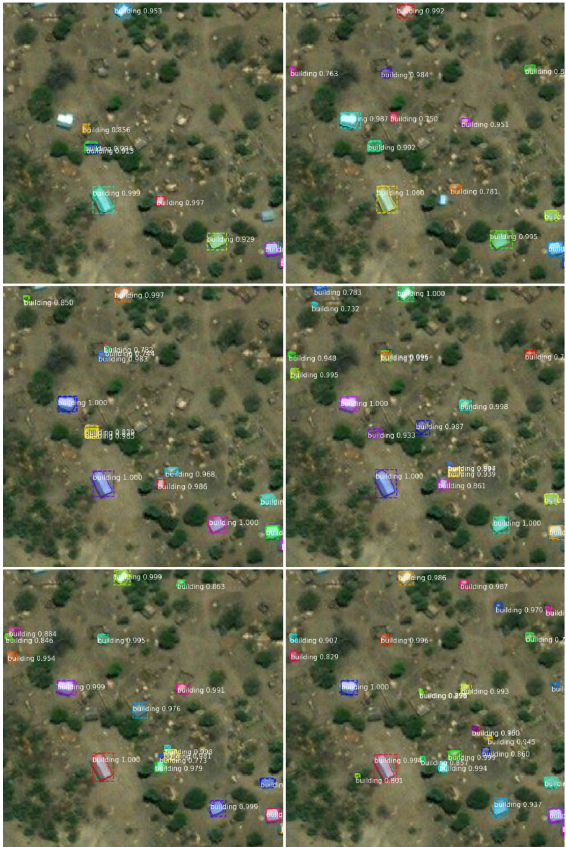
Figure 5.3: Mask R-CNN predictions on different upsampling scales. From left to right and top to bottom the upsampling ratios are 2, 3, 4, 5, 7 and 10 respectively.
