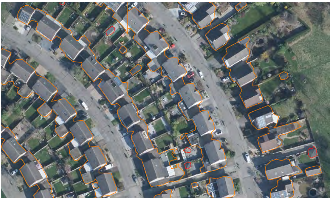
Figure 6.12: Vectorized predictions on Heerlen. An orange outline indicates the prediction overlaps at least one building in the ground truth, red indicates no overlap.
