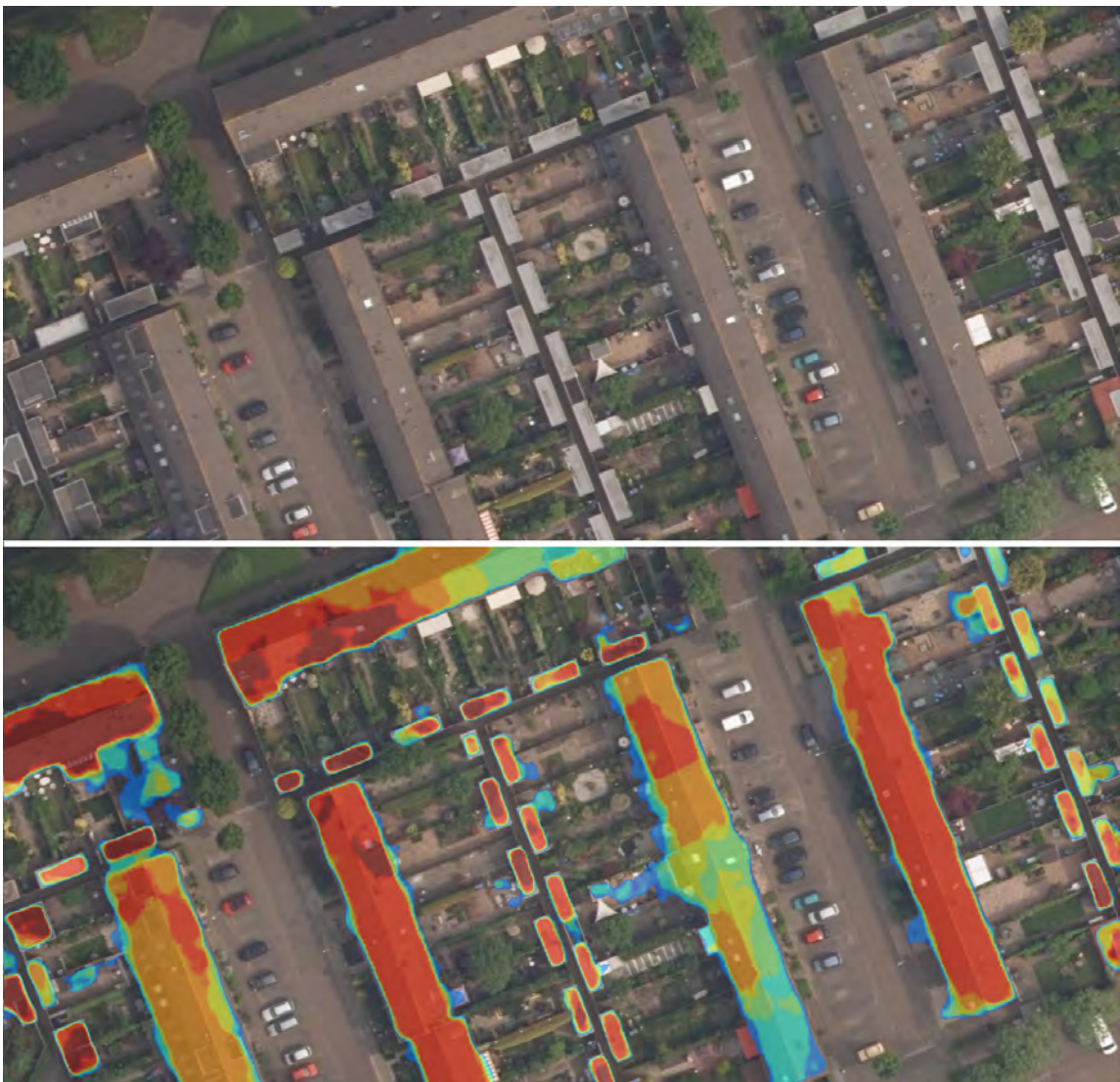
Figure 6.1: Top: Sample image of 153.6 by 72.2 meters from the test set showing the Amersfoort municipality at 10 cm resolution. Bottom: TTA ResU-net predictions inferred on imagery downsampled to 30 cm resolution but plotted over the original 10 cm imagery. A darker red color indicates a higher predicted probability of the underlying pixel being a building. Only predictions above a 0.2 probability are plotted.
