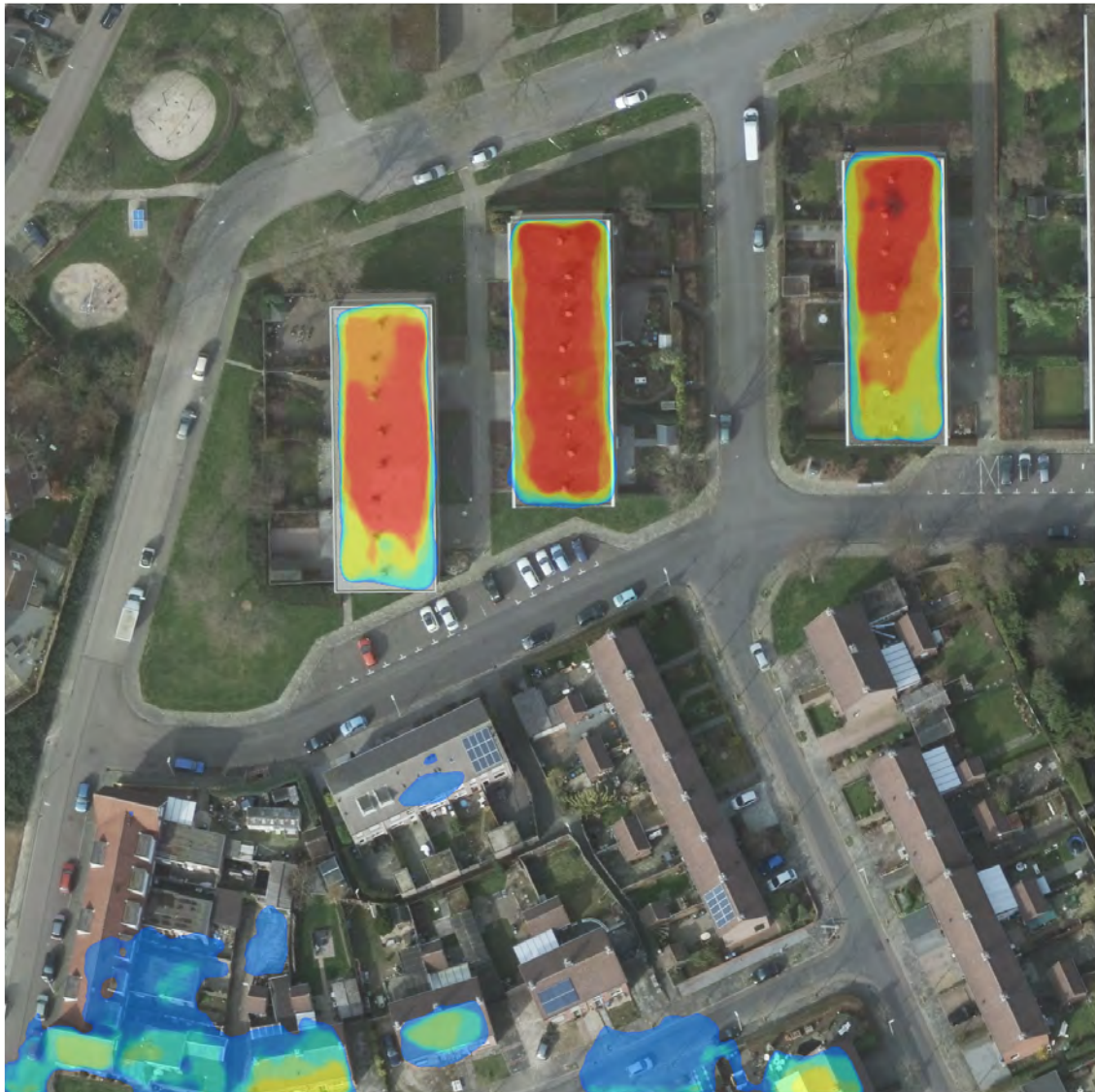
Figure B.12: TTA predictions of ResU-net resolution robustness experiment 3: Trained on 10 cm resolution imagery, tested on 30 cm resolution imagery of Heerlen, The Netherlands. Plotted on 10 cm imagery.
