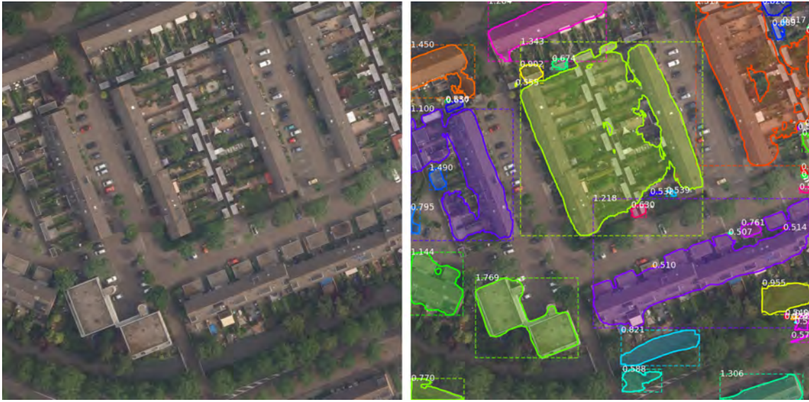
Figure 5.9: Left: Sample of 153.6 by 153.6 meters from imagery of Amersfoort at 10 cm resolution. Right: TTA predictions of Mask R-CNN on the sample image downsampled to 30 cm, plotted on the original 10 cm imagery.
