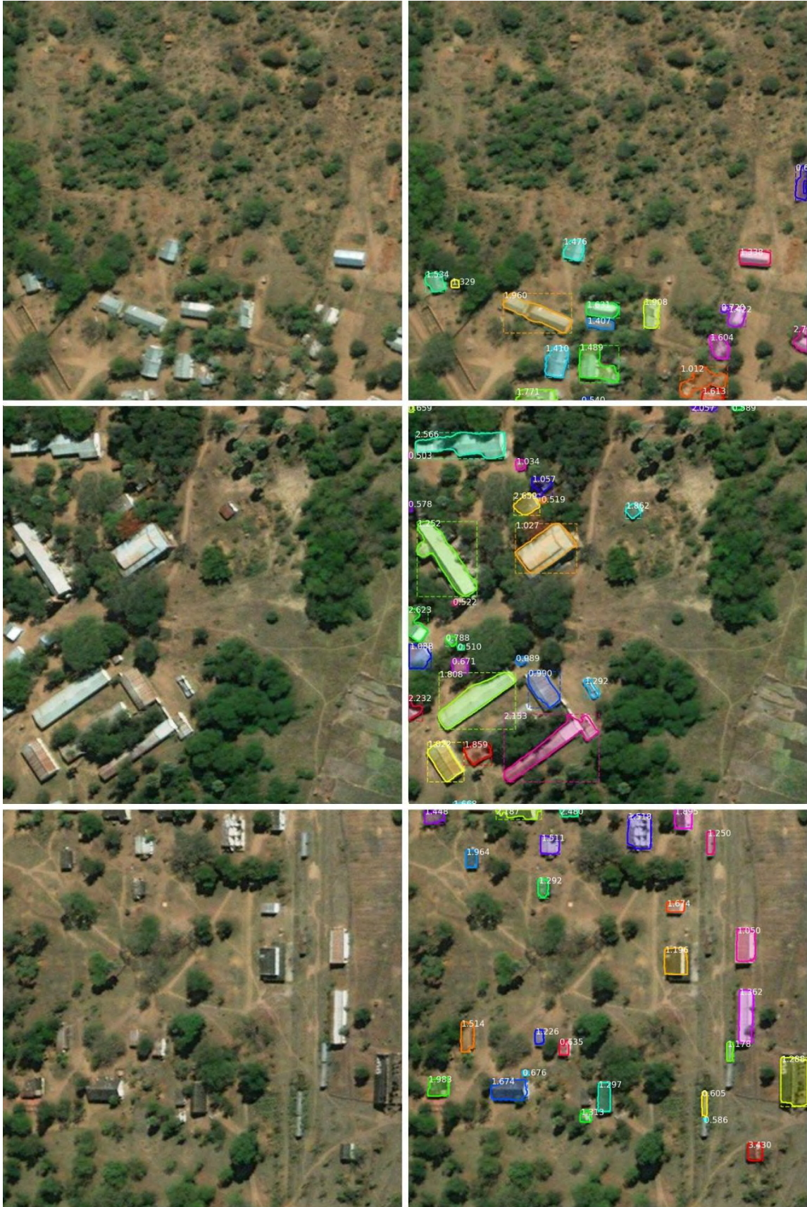
Figure 5.4: Left: Samples of 230.4 by 230.4 meters from imagery of Nsanje at 30 cm resolution. Right: TTA predictions of Mask R-CNN on imagery upsampled by a factor of 2.5.
