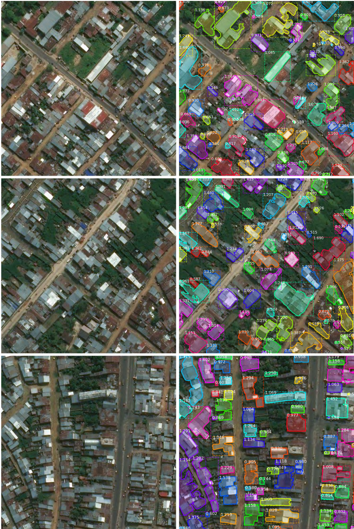
Figure 5.7: Left: Samples of 230.4 by 230.4 meters from imagery of Equitos at 30 cm resolution. Right: TTA predictions of Mask R-CNN on the original imagery.
