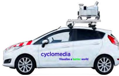
Figure 3: Setup used to capture the point cloud.
