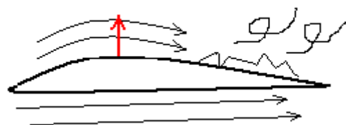
Figure 3: Ice on the wings disturbs the airflow reduces the pressure difference above and below the wing. This causes the lift to be smaller at a certain velocity.
