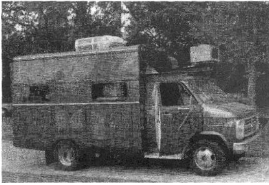
Fig. 3. The Carnegie Mellon NAVLAB autonomous navigation testbed.
