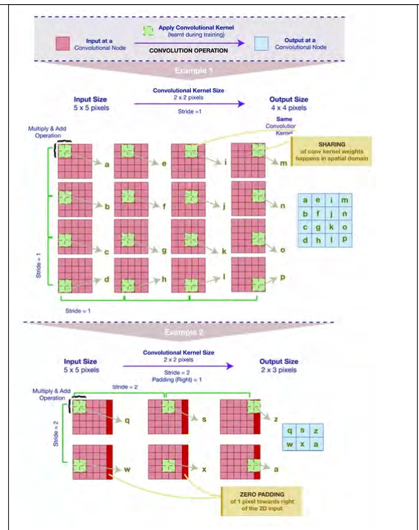
Fig. 4. How a feature map is created in a convolution or max pooling layer [41].
